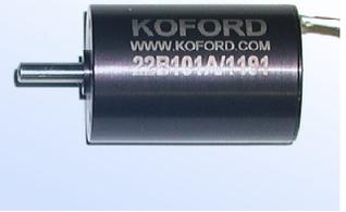
These motors are suitable for use with sine drives and exhibit exceptionally smoothness when driven by encoder controlled sinusoidal drives. Custom versions including, hollow shafts, frameless, can be provided. Application include actuators, miniature servo systems, filter wheels, medical pumps, and blowers
