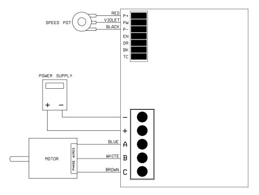
Stand alone operation with speed pot, motor direction can be reversed by switching Blue and White leads
