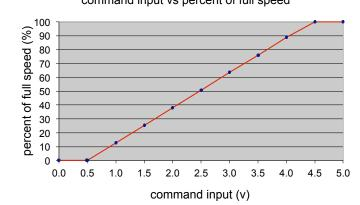
H48V20A - A6 command input vs speed
