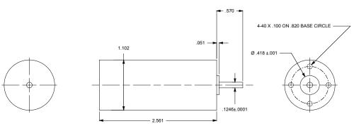
Leads are 12" minimum Phase leads are 24 gauge, hall leads are 28 gauge, all TFE insulation
