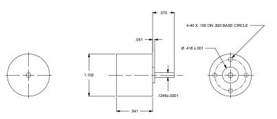
Leads are 12" minimum Phase leads are 24 gauge, hall leads are 28 gauge, all TFE insulation
