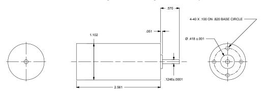
Leads are 12" minimum Phase leads are 24 gauge, hall leads are 28 gauge, all TFE insulation
